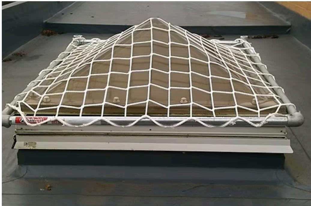
The Safetube system consists of a galvanised tubular frame, being easily assembled on site. These are simply placed over the fragile roof area often requiring no fixings into the roof structure, and can also be used by operatives when carrying out site surveys in addition to longer term protection.
